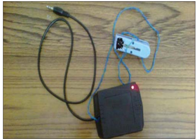
Figure 1: Digital finger pulse photoplethysmography
